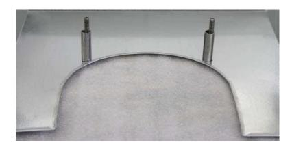
5. Tighten the bolts with a 7/16" wrench.
